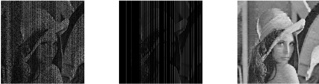
(b) Norm sampling (without replacement). Selection error \|\mathbf{M} - \mathbf{C}\mathbf{C}^\dagger\mathbf{M}\|_F / \|\mathbf{M}\|_F = 0.106 .
